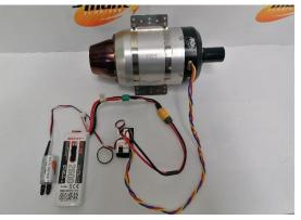
LiFe battery of 9,9V /25C, although the engine run better with the recommended Lipo battery. Other battery voltages are not supported. **Battery should be connected directly, DO NOT use switches** (electronic or mechanical), electronic regulators, diodes, voltage regulators, etc. Multiple battery operation using a "Y" lead is possible, but at least one battery must be directly connected to the ecu.
