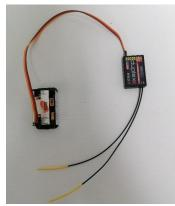
supported. **Battery should be connected directly, DO NOT use switches** (electronic or mechanical), electronic regulators, diodes, voltage regulators, etc. Multiple battery operation using a "Y" lead is possible, but at least one battery must be directly connected to the ecu.
