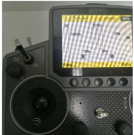
On some Futaba transmitters, it has been found that the throttle channel the sense of movement may require reversing (Servo reverse) and to repeat the transmitter alignment. The correct adjustment of the throttle adjustment on the ecu can be verified in the second screen of the data terminal, the percentage of the throttle position should read 0% at the position of engine stop (trim and stick down), 100% with stick/trim full up and between 10% and 30% at idle.
