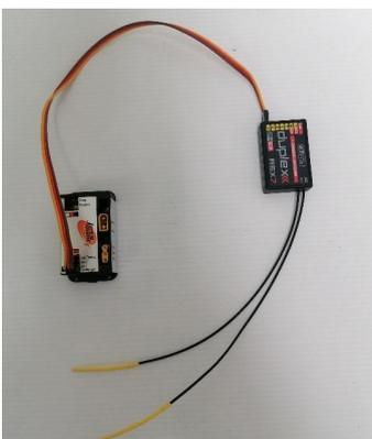
LiFe battery of 9,9V /25C, although the engine run better with the recommended Lipo battery. Other battery voltages are not supported. **Battery should be connected directly, DO NOT use switches** (electronic or mechanical), electronic regulators, diodes, voltage regulators, etc. Multiple battery operation using a “Y” lead is possible, but at least one battery must be directly connected to the ecu.
