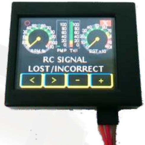
Data, including all engine parameters, can be saved later to a memory card, where it can be read using a text editor, or our viewer software. Also can be sent to engine manufacturer to be studied, and changes uploaded back to the ecu.
