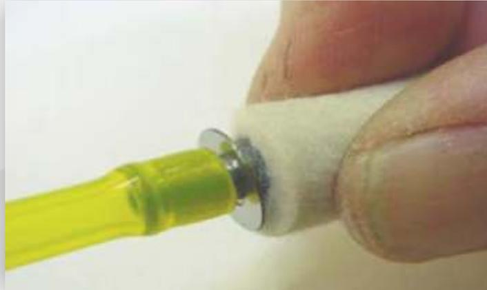
A BVM UAT is another contemporary method of reducing the possibility of air bubbles in the engine fuel line. This is a very important aspect of the operation of any turbine engine. Use an appropriate adapter for the 6mm tube output of the UAT to the 4mm in the inlet side of the fuel pump, direction of fuel flow is clearly shown at the top of the pump. The clear 4mm tubing is used on the pressure side of the pump.
