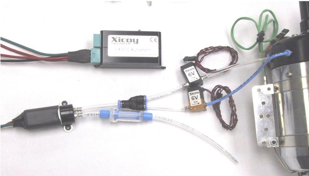
Install the fuel system components as seen in the picture.
