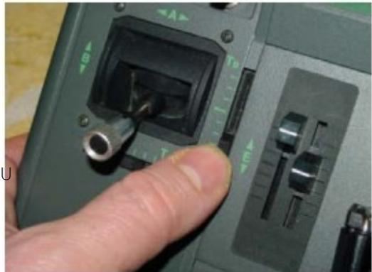
When using a Futaba transmitter, the throttle channel sense of movement may require reversing (Servo reverse) and if so reverse and repeat the transmitter alignment. Correct reading of throttle % by the ecu can be verified in the second screen of the HDT, percentage of the throttle position is shown on, 0% in the position of engine stop (trim and stick down), 100% with stick/trim full up and between 10% and 30% at idle.
