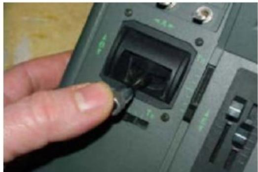
Leaving the throttle stick in the minimum position, raise the throttle trim to the full up position or switch "Engine Cut" switch to off, and again press the "+" button to store the value into the ecu.
