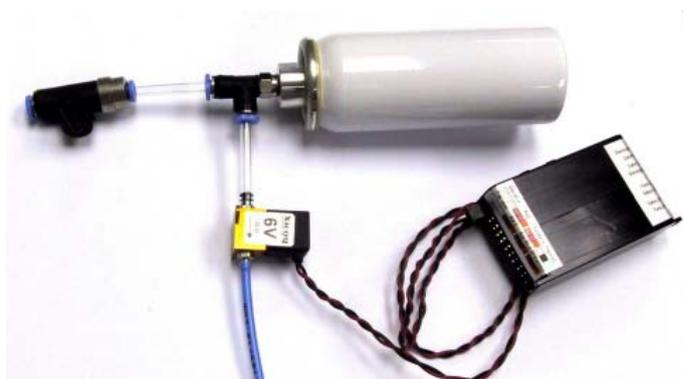
The Merlin starting gas system can use any suitable size of easily available gas canister, available from most camping/outdoor stores or DIY outlets. A suitable on/off tap should be secured to the canister, then fed to the inlet side of the gas valve via a suitable length of 4 mm plastic tubing.
