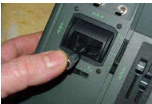
Leaving the throttle stick in the minimum position, raise the throttle trim to the full up position or switch "Engine Cut" switch to off, and again press the "+" button to store the value into the ecu.
